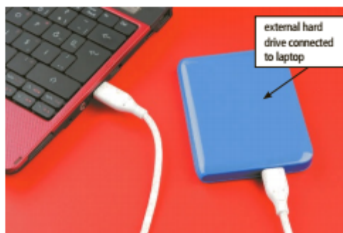
Figure 1-22 A external hard drive is a separate, freestanding storage device.
