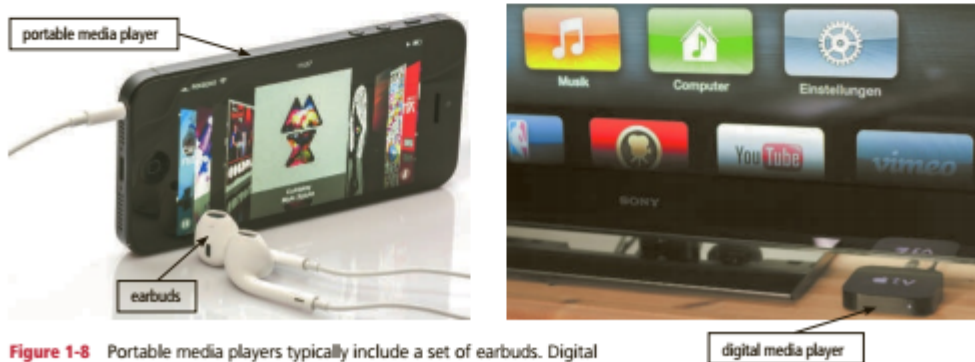
Figure 1-8 Portable media players typically include a set of earbuds. Digital media players stream media to a home entertainment device.
