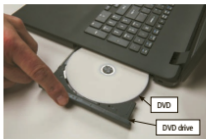
Figure 1-25 You can insert a DVD in a DVD drive on a computer. Some computers have DVD slots instead of DVD drives.
